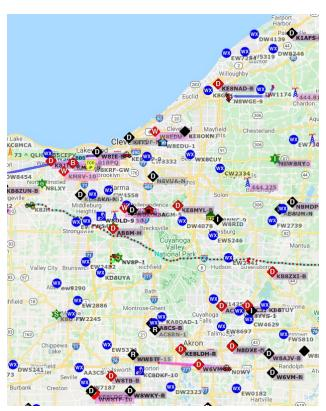
Automatic Packet Reporting System (APRS) is an amateur radio-based system for real time digital communications of information of immediate value in the local area. Data can include object Global Positioning System (GPS) coordinates, weather station telemetry, text messages, announcements, queries, and other telemetry. APRS data can be displayed on a map, which can show stations, objects, tracks of moving objects, weather stations, search and rescue data, and direction finding data.
