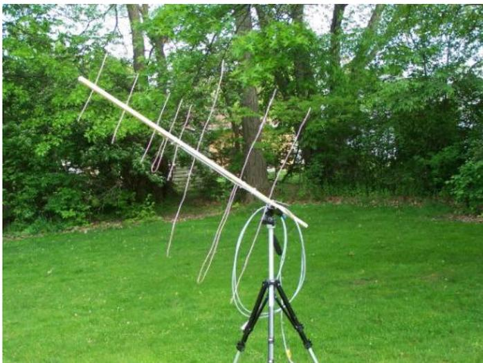
bare copper wire. The total cost of the antenna itself came in under \$20. Throw in some coax assemblies, a PVC tee and some hardware for the camera tripod mount and the whole thing costs less than \$50, ready to use.
